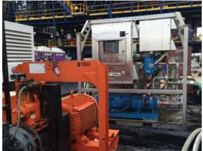
*ICU 150 with 6 x 6 Centrifugal Pump on Deck*
