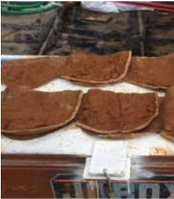
*BEFORE: Initial Flush Filtration Bag Inspection on Heat Medium Piping System*
