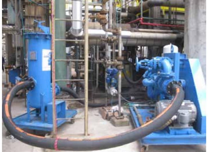
*Flushing skid with positive displacement pump at 500 GPM flow and filter housing with four 34" filter elements.*
