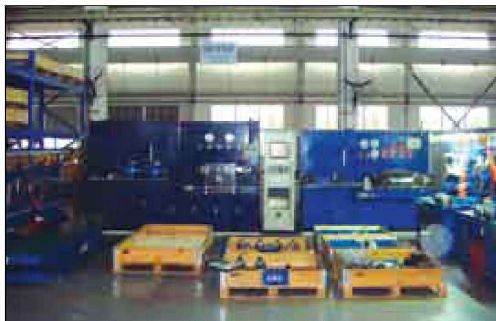
Test benches for Imo three-screw pumps
