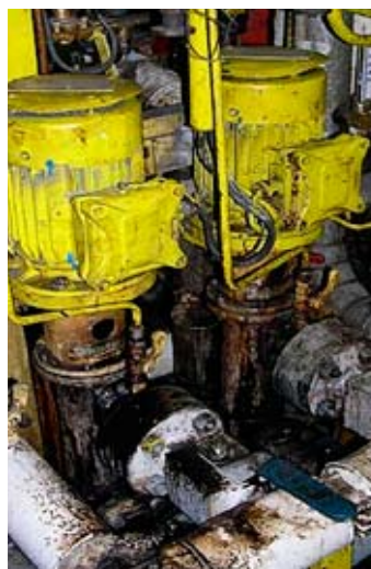
Left: Stena Danica’s old mechanically sealed pump. Right: Spring 2008 – Stena Danica’s new IMO OptiLine pumps.
