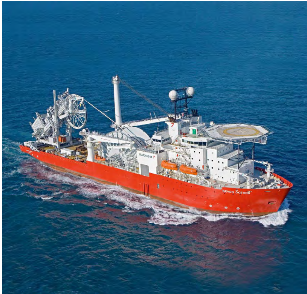
IHC MERWEDE Shipyard, Reeled Rigid Pipe-Laying – Offshore Construction Vessel „SEVEN OCEANS“ equipped with ALLWEILER Solutions.
